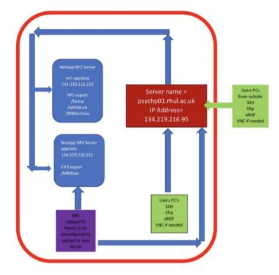
Red outer line indicates VPN. Users from home are given firewall access so that they can connect to the server using SSH, SFTP, xRDP and VNC protocols.
